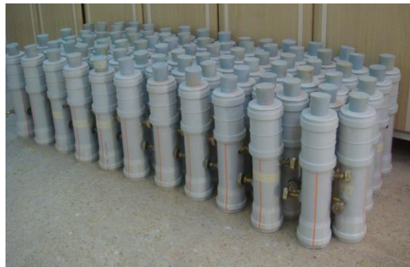
Figure 3: Radon and thoron chambers construction exhalation rate .
