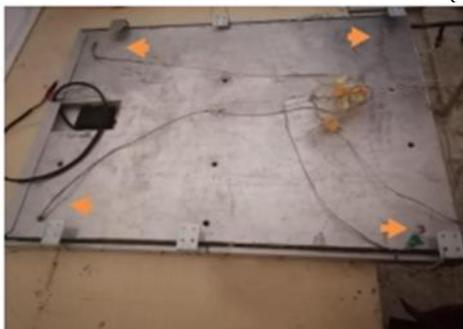
(b) Thermocouples location on the plate heat exchanger
