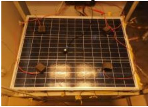
(a) Sensor of Solar Meter, Insolated thermocouples and connected rods of Digital Multimeter
