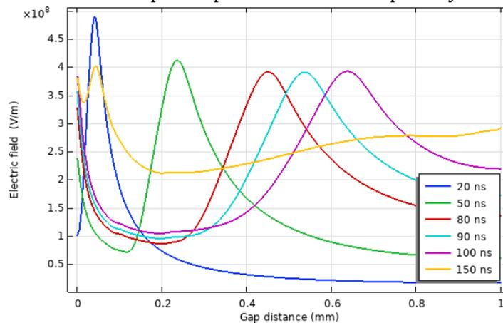
**Table 3.** the evolution of the streamer in the rod-plate system at a different time scale and the applied voltage was fixed at 300 kV.
