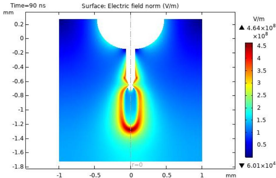
**Figure 5.** A streamer discharge's growth in transformer oil at 300 kV for the needle-plate electrode.
