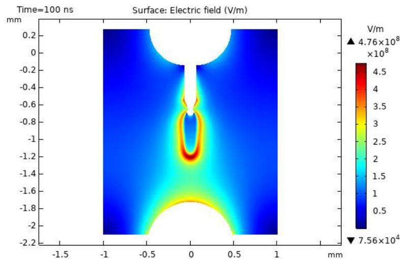
**Figure 10.** The evolution of a streamer discharge in transformer oil at 300 kV of applied voltage for the needle-sphere electrode.
