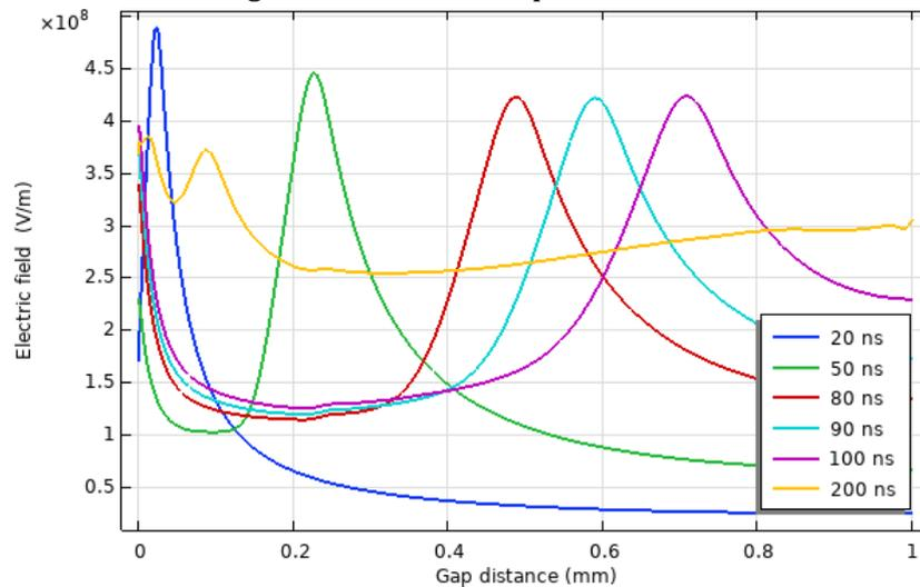
**Table 2.** The evolution of the streamer in the needle-plate system at a different time scale and the applied voltage was fixed at 300 kV.
