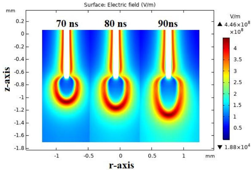
During this study, we noticed that the lowest voltage to achieve a transition to the third from the second mode was (265 kV) at the time (100 ns) for a rod-plate electrode. Table 2 the evolution of the streamer in the rod-plate system at a different time scale and the applied voltage was fixed at 300 kV. The electric field can be represented for some time phases in one dimension, the stages of the streamer are as shown in the figure below for the rod-plate system.
