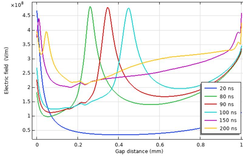
**Table 4.** the evolution of the streamer in the Needle-sphere system at a different time scale and the applied voltage was fixed at 300 kV.
