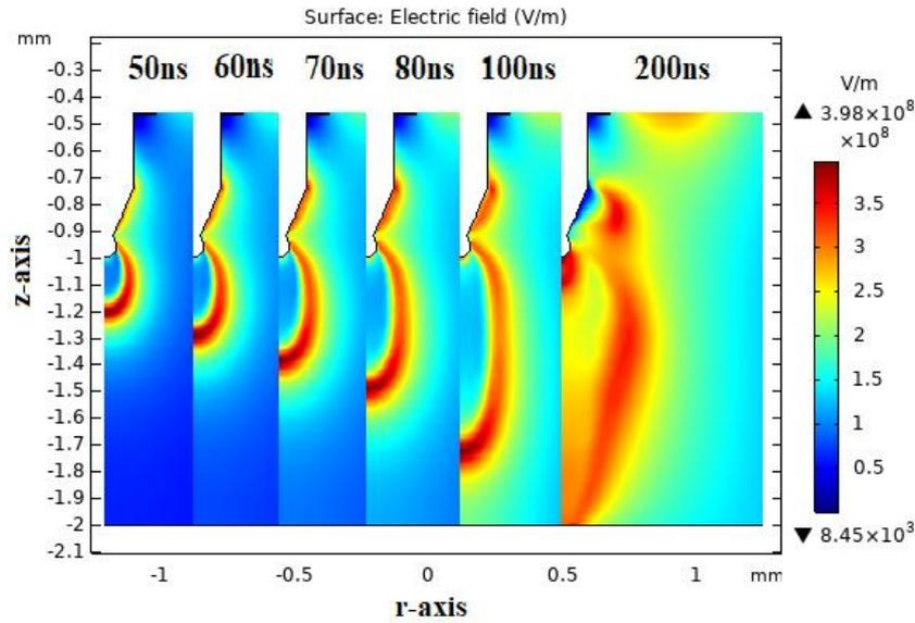
In Table 1 below, the values obtained during the simulation process, the values show the evolution of the streamer in the needle-plate system and the change from the 2<sup>nd</sup> to the 3<sup>rd</sup> mode according to the velocity of the streamer discharge through the transformer oil. Figure 6, represents the change in the shape of the streamer according to the periods shown in the one-dimensional diagram.
